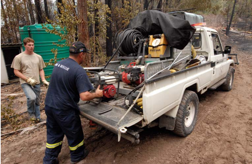
A landowner's vehicle, fitted with fire fighting equipment
