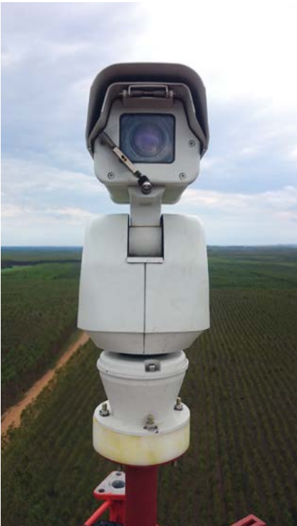
The Firehawk wildfire detection camera scans a full 360 degrees in under four minutes
